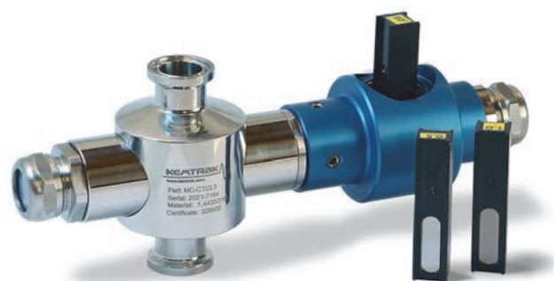
Figure 12) Kemtrak 3/4" Tri-Clamp type in-line measurement cell with validation accessory using certified filters in a standard 12.5 mm size cuvette format
