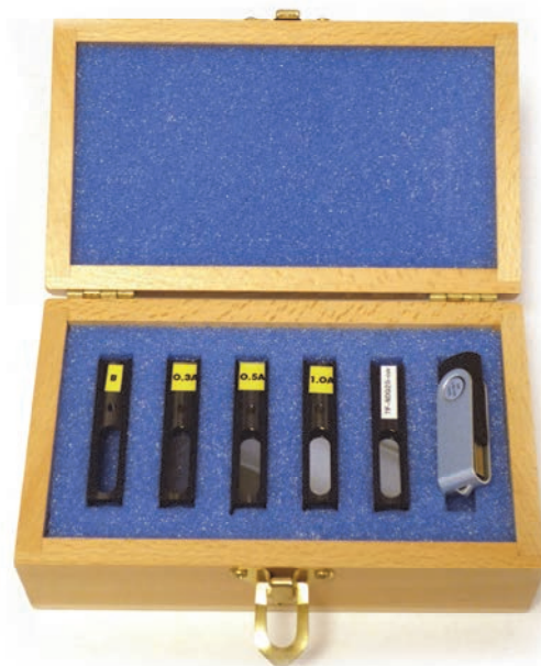
Figure 11) NIST traceable metal on fused silica glass absorption filter set for 12.5 mm standard cuvette holder
