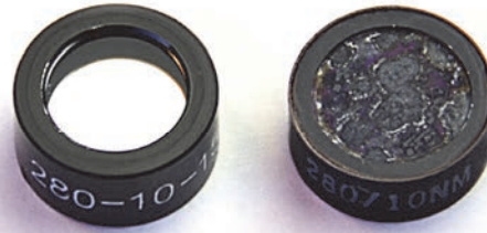
Figure 8) Bandpass filter damage. New filter is shown on the left, eroded optical filter due to prolonged exposure to a hot mercury type UV lamp on the right.
